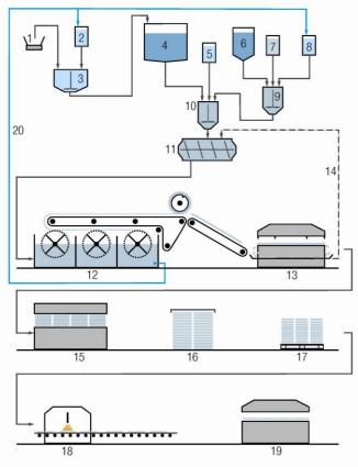
1 Scales for process fibres (pulp) 11 Horizontal mixer 2 Water 12 Platen machine 3 Pulper 13 Punching machine 4 Vat process fibres in water 14 Punching sections 5 Reinforcing fibres (synthetic fibres) 15 Press 6 Portland cement 16 Setting 7 Admixed substances 17 Half-finished products' warehouse 8 Water 18 Coating 9 Intensive mixer 1 19 Punching 10 Intensive mixer 2 20 Water cycle
