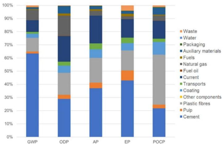
The environmental impact of the pulp in the base mix is relevant only in the eutrophication potential (EP). The share of the total load for this indicator is 8%. The influence of the coating is greatest at the formation potential for tropospheric
