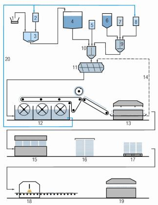
1 Scales for process fibres (pulp) 11 Horizontal mixer 2 Water 12 Platen machine 3 Pulper 13 Punching machine 4 Vat process fibres in water 14 Punching sections 5 Reinforcing fibres (synthetic fibres) 15 Press 6 Portland cement 16 Setting 17 Half-finished products' warehouse 7 Admixed substances 8 Water 18 Coating 9 Intensive mixer 1 19 Punching 10 Intensive mixer 2 20 Water cycle
