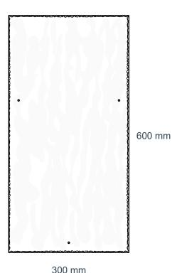
manufactured in accordance with the requirements of the European Norm EN 492. They have achieved Class B, the highest class, for structural stability in accordance with EN 492.
