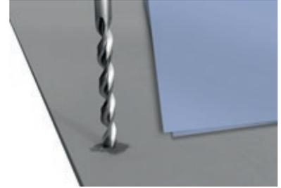
If not using Swisspearl Facade Wing Screws, the boards should be pre-drilled with an appropriate fibre cement drill bit. Dust from cutting or drilling must be removed with a brush or a fiber cloth immediately after the work has been completed, otherwise it can mark the surface of the boards.
