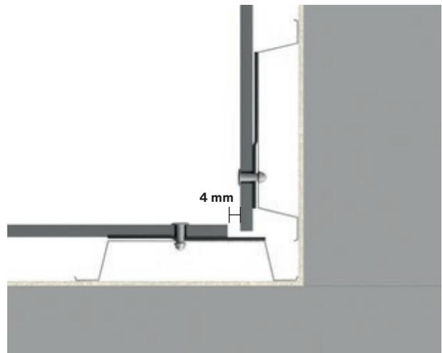
Horizontal view: Internal corner construction with open joint
