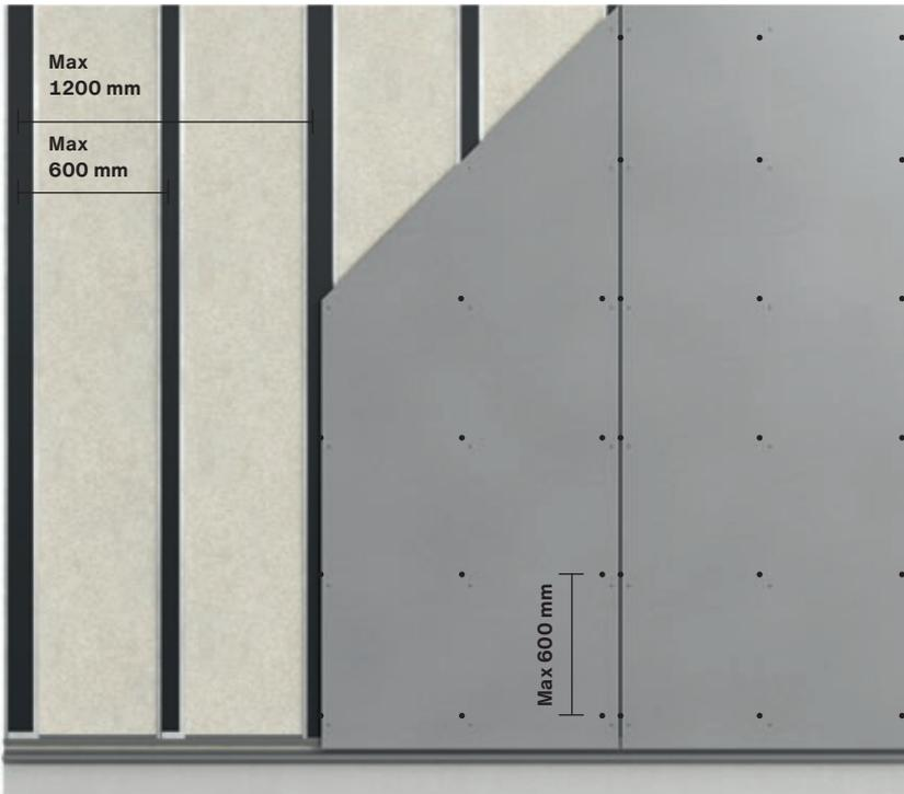
Swisspearl facade boards installed on vertical VFL profiles
