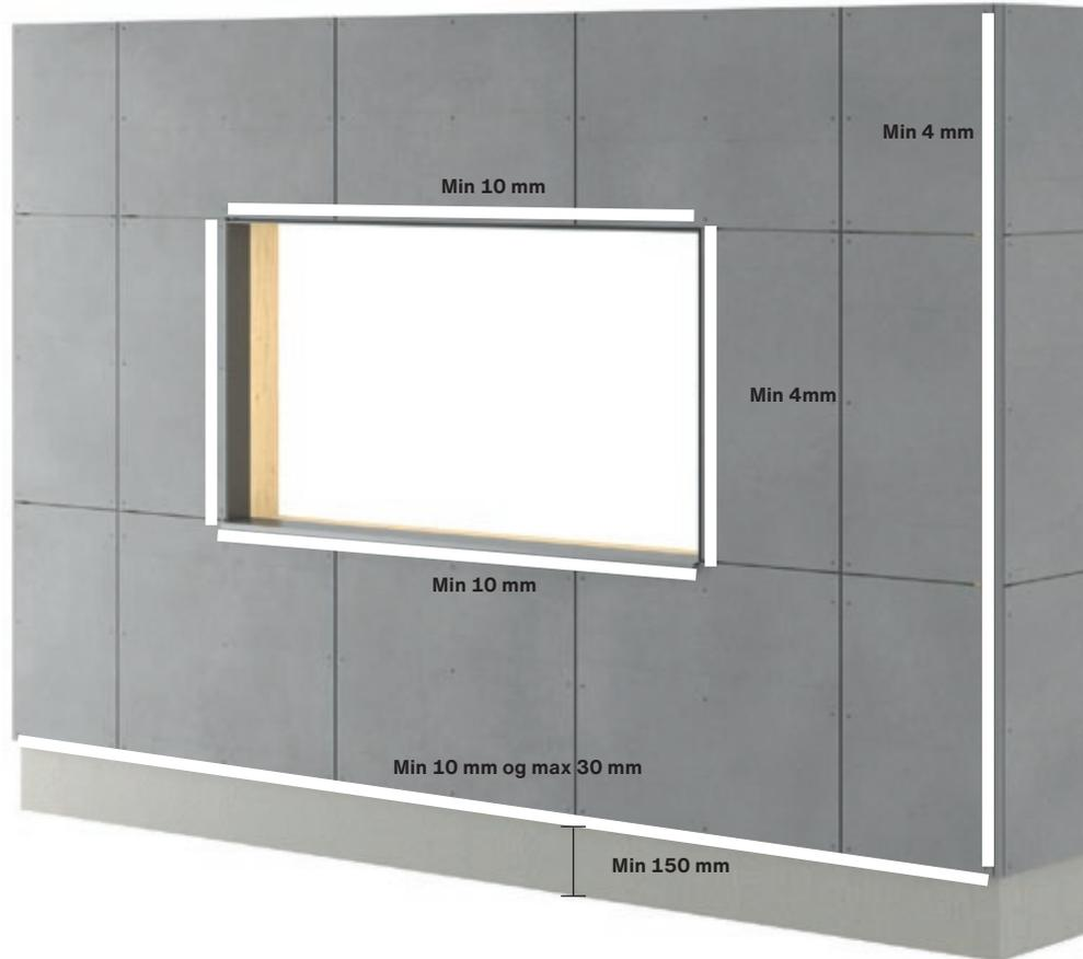
Follow the guidelines regarding distances described in this manual. The facade board should finish between 10 and 30mm below the bottom end of the substructure. For overhang and similar, the maximum distance is 100mm.
