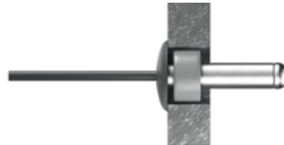
X : Fixing position hole diameter  $\varnothing 9$  mm.
