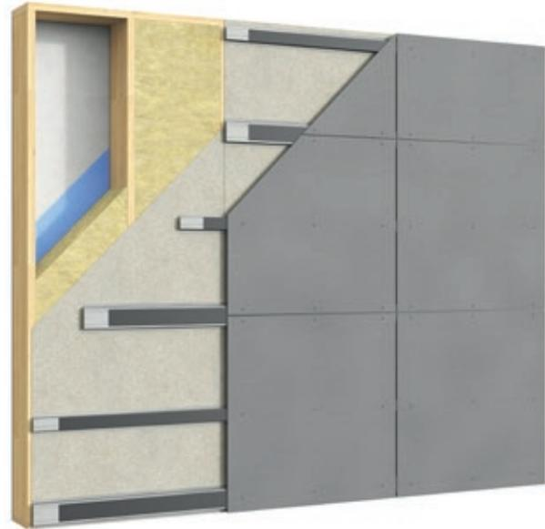
Light wall with horizontal VFL steel profiles
