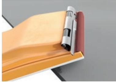
Once boards are cut, you can bevel the cut edge with a fine grinder (80 grain) to give the edge a pre-cut finish. The bevel should be angled at 45° relative to the board. This retains edge strength and removes small irregularities.
