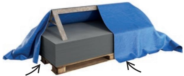
Replace the plastic with a tarpaulin. It is very important that there is ventilation all around the tarpaulin and also on top of the pallet under the tarpaulin. This is done to make sure that condensation is reduced as much as possible.
