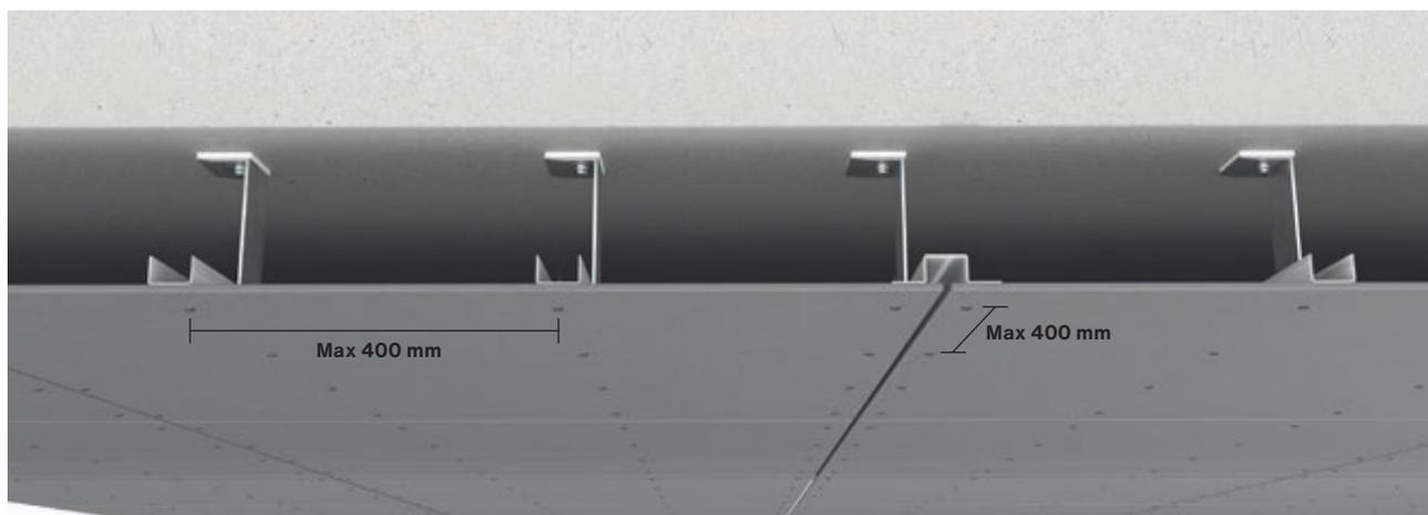
When using Swisspearl facade boards as ceiling or soffit, you can normally use a regular steel system with steel profiles, but for larger cavities, you need to contact a steel manufacturer to make sure the system fits your needs. The number of brackets and types of anchoring used for the type of deck/ceiling has to be calculated, and the manufacturer's instructions should always be followed.
