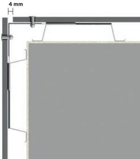
Horizontal view: External corner construction with open joint
