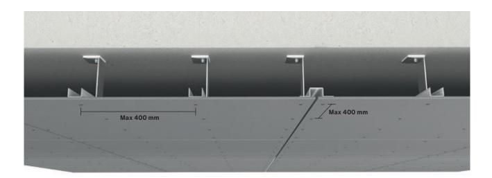
When using Swisspearl facade boards as ceiling or soffit, you can normally use a regular steel system with steel profiles, but for larger cavities, you need to contact an steel manufacturer to make sure the system fits your needs. The number of brackets and types of anchoring used for the type of deck/ceiling has to be calculat-ed, and the manufacturer's instructions should always be followed.
