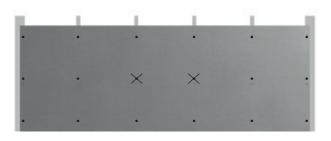
Example: Horizontally mounted boards with four intermediate steel profiles
