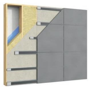
Light wall with horizontal VFL steel profiles
