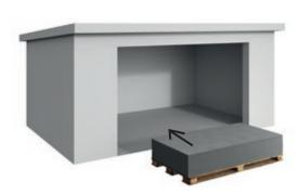
If Swisspearl facade boards are stored more than 2-3 weeks on site, the pallets should be kept under a roof to ensure dry and ventilated conditions.
