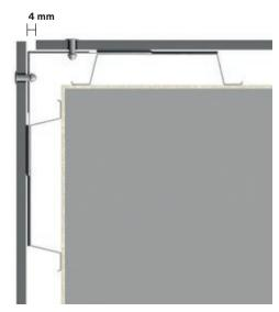
Horizontal view: External corner construction with open joint It is possible to create an external corner detail without a Swisspearl corner profile. There should be a min. 4mm gap between the facade boards forming the corner joint. If using brackets and profiles, an angle profile can be used behind the facade. It should be fixed with screws or rivets. The distance from the corner to the profile that is fixed to the wall should not be more than 200mm.
