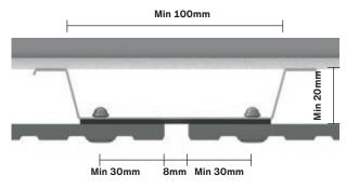
Fig. 1. Swisspearl Patina Inline installation on profile behind joint.
