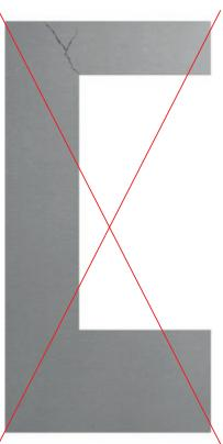
Fig. 3. Incorrect installation of Swisspearl facade boards at windows, doors and openings.
