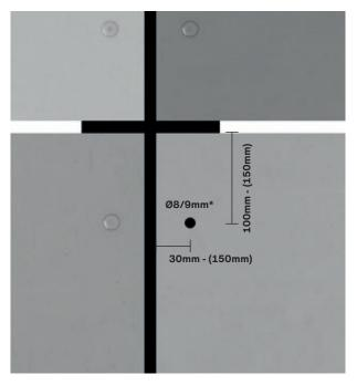
Example of vertical substructure
