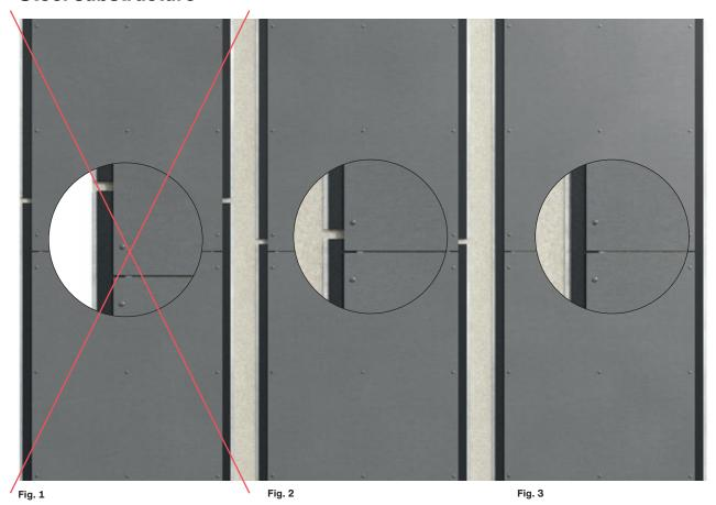
Correct installation of the steel support system Never install Swisspearl facade boards spanning over two or more steel profiles lengthwise, as movement of the steel and the facade boards caused by mois-ture and temperature changes potentially could damage the boards (fig. 1).
