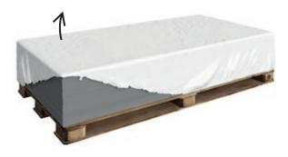
If the pallets are stored outside when they arrive at the building site, the plastic cover should be removed. The facade boards should be stored on the pallet or sleepers with max 500mm distances.
