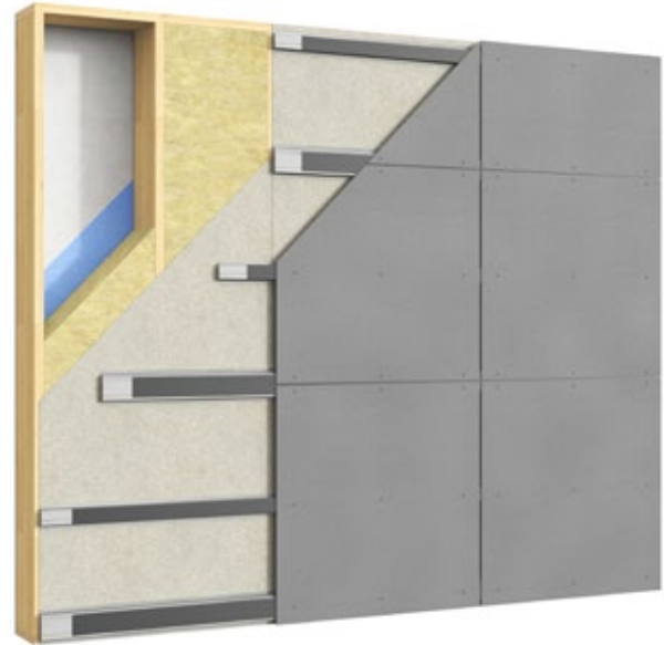
Light wall with horizontal VFL steel profiles
