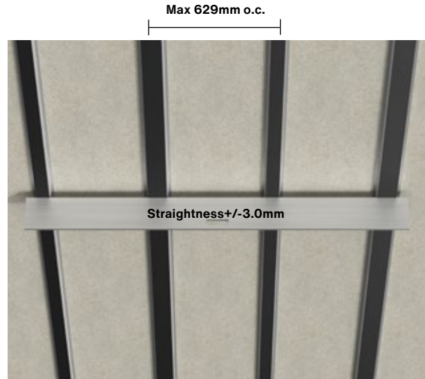
Straightness of substructure
