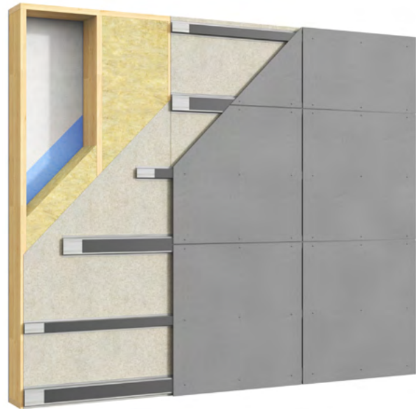
Light wall with horizontal VFL steel profiles
