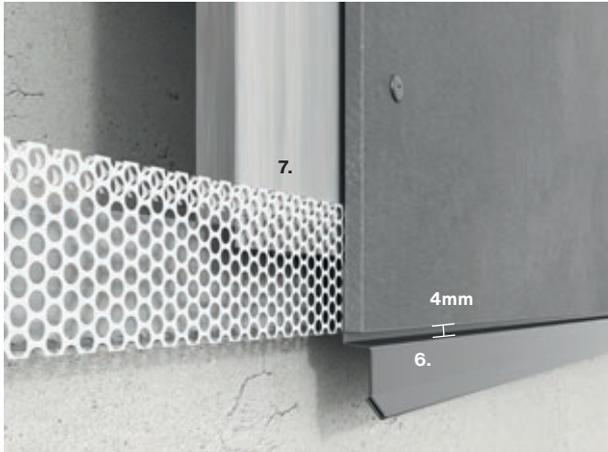
Swisspearl Drip Small is used to drain water away from the supporting structure or where neat detailing is required at the foot of the facade.
