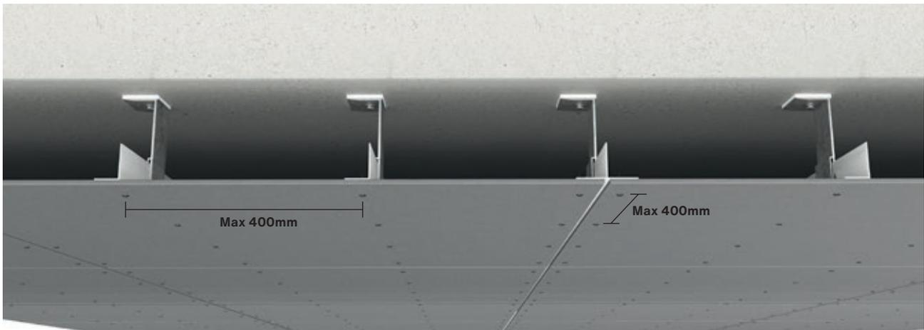
When using Swisspearl facade boards as ceiling or soffit, you can normally use a regular aluminium system with brackets and T and L profiles, but for larger cavities, you need to contact an aluminium manufacturer to make sure the system fits your needs. The number of brackets and types of anchoring used for the type of deck/ceiling has to be calculated, and the manufacturer's instructions should always be followed.
