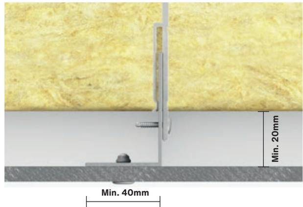
To ensure that boards are able to accommodate movement without damage, please adhere to the following Swisspearl guidelines for correct fixing centres and hole sizes.
