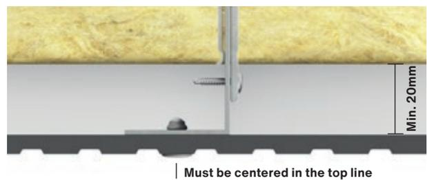
Fig. 2. Swisspearl Patina Inline installation on L profile.
