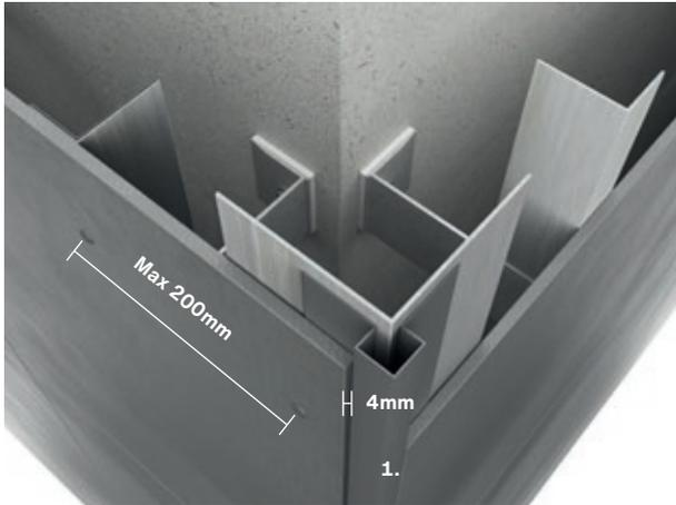
Swisspearl External Corner Small is used for 90° external corner constructions, to create a securely finished detail. Use double sided tape to temporarily fix the profile to the facade board before fixing it with rivets. Make sure the correct edge distances and hole sizes are used. The distance from the corner edge to the wall T or L profile should not exceed 200mm. There should be a minimum 4mm gap between the board edge and the profile.
