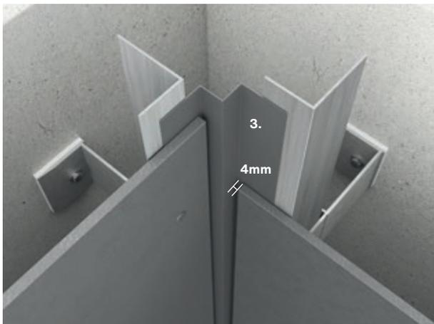
Swisspearl Internal Corner is used for 90° internal corners. Secure the profiles with double sided tape. Once fixed, the facade board will secure the profiles in position. There should be a minimum 4mm gap between the board edge and the profile.
