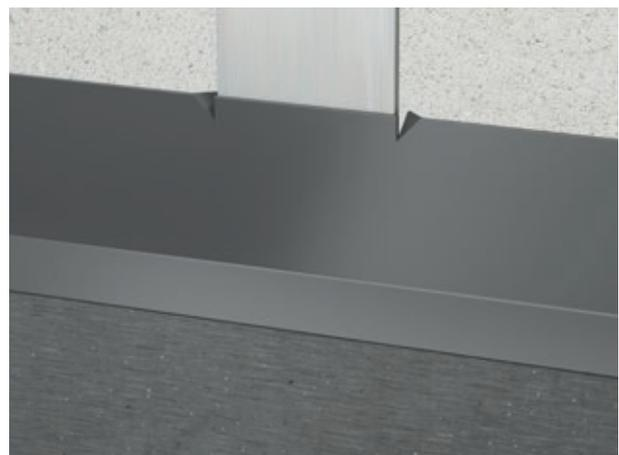
It may be useful to cut and fold out a triangle in the horizontal profile on each side of the vertical T- or L-profile, as shown in the illustration. This will prevent the horizontal profiles from moving.
