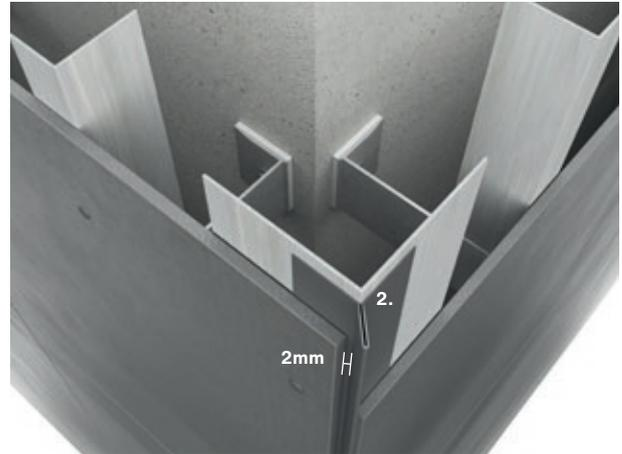
Swisspearl External Corner Peak can also be used for 90° external corner constructions. It is installed in the same way as Swisspearl External Corner Small. The distance from the inside edge of the facade boards to the profile should be a minimum of 2mm.
