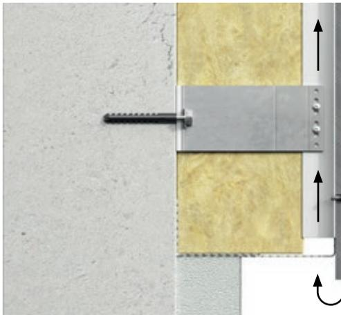
Air is pulled into the construction through an opening at the base of the facade, and it must be ensured that unobstructed ventilation is possible throughout the facade's height. There should be a ventilation gap of minimum 10mm, or equivalent 100cm<sup>2</sup> per meter. If perforated profiles are used, a ventilation area opening of minimum 100cm<sup>2</sup> per meter is required. The opening at the base is also used to drain moisture that has entered the facade.
