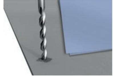
If not using Swisspearl Facade Wing Screws, the boards should be pre-drilled with an appropriate fibre cement drill bit.
