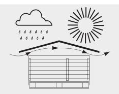
Stacks must be stored out of dampness and direct sunlight. The polythene cap, the Profile 8 are supplies in, is not sufficient!
