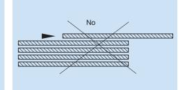
Wrong Panels shall not be pulled from the stack
