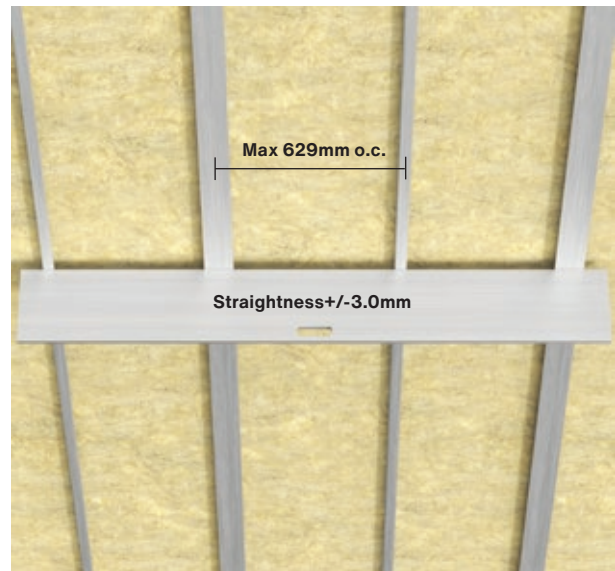
Straightness of substructure
