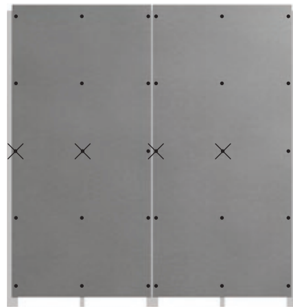
Example: Vertically mounted boards with one intermediate aluminium profile
