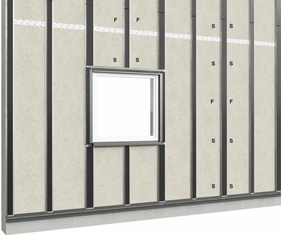
Fixing points (F) Sliding points (S)
