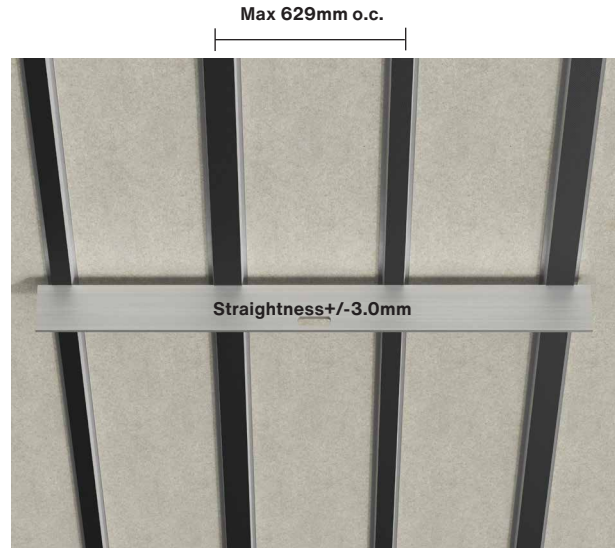
Straightness of substructure
