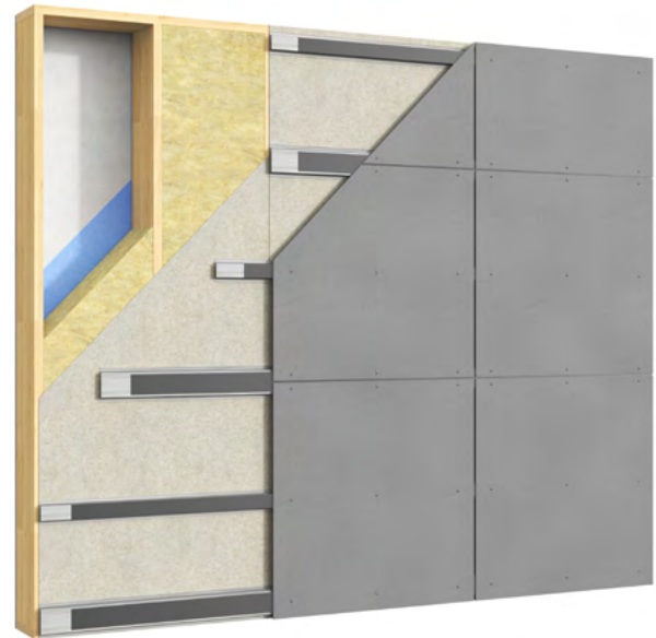
Light wall with horizontal VFL steel profiles
