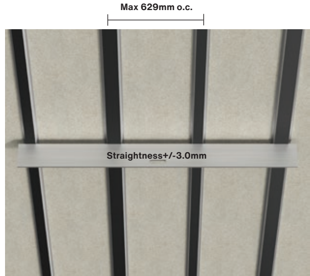
Straightness of substructure
