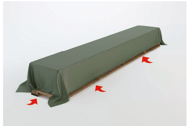
Important: Store materials under a dry and well-ventilated tarpaulin. If the product becomes damp, it should be placed on its vertical edge to allow rapid drying. Never install wet products.
