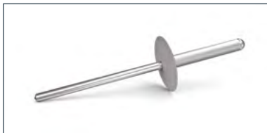
Swisspearl Rivets Aluminium RIV-A EPDM Washer 4.0x20mm Aluminium body and Stainless steel mandrel. Unpainted or colour coated to the facade boards Grip Range 11-15mm
