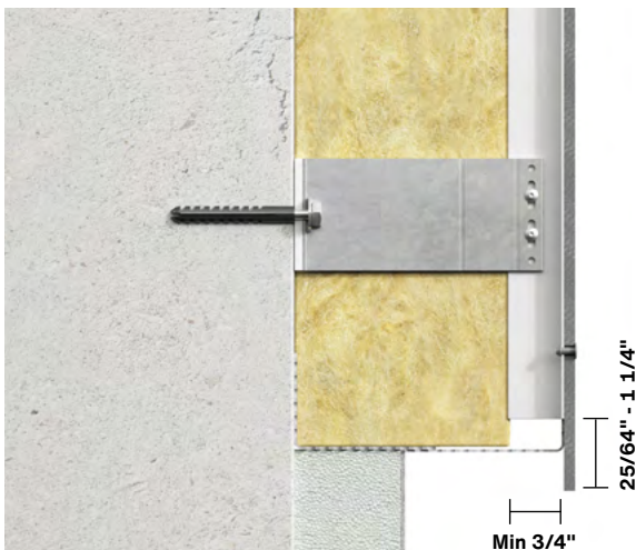
Vertical view: Plinth construction
