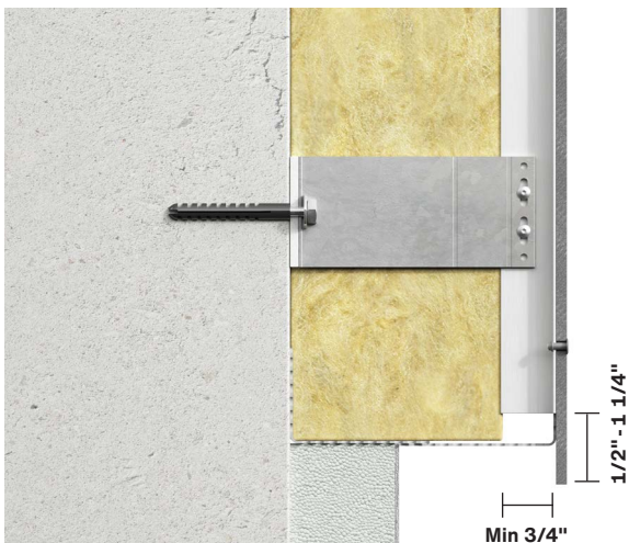
Vertical view: plinth construction
