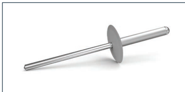
Swisspearl Rivets Aluminum Swisspearl aluminum rivet head Ø15 mm, blank or powder-coated. 4.0x18-K15, 8-13 mm grip range
