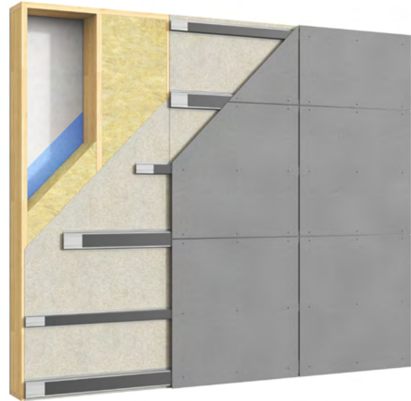
Light wall with horizontal steel profiles
