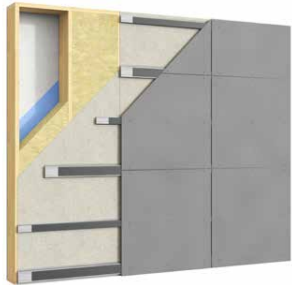
Light wall with horizontal steel profiles
