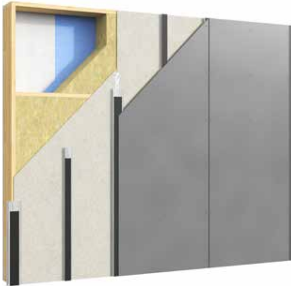
Light wall with vertical steel profiles
