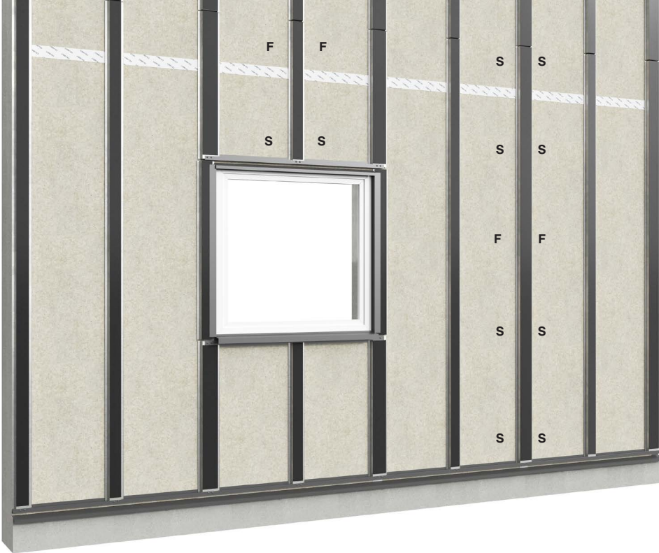
Fixing points (F) Sliding points (S)
