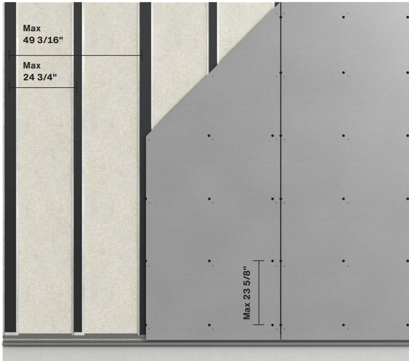
Swisspearl facade boards installed on vertical VFL profiles
