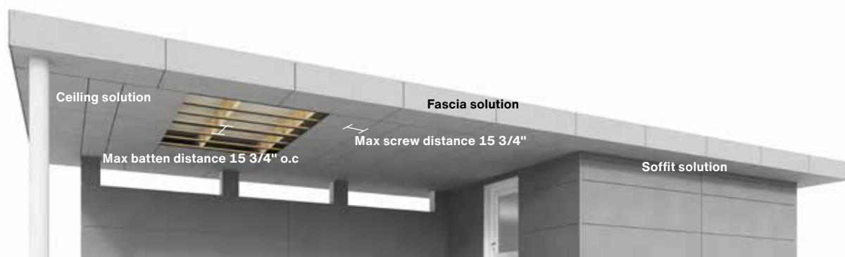
Screw and batten distances
