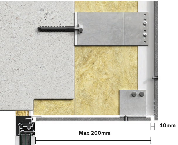
Vertical view: Window head As with jambs, the window head can be formed using Swisspearl boards. At the front edge of the head detail, ensure a minimum free opening area of 20mm, or equivalent 200cm 2 per meter to ensure adequate ventilation behind the facade. If ventilation profiles are used, the perforated opening area must correspond to min. 60% of the opening area.
