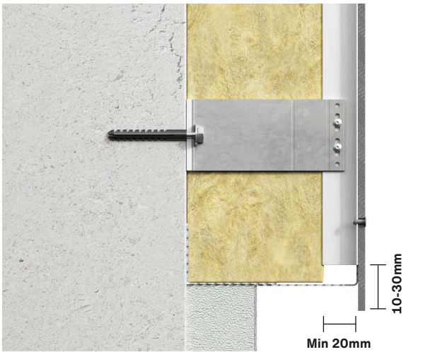
Vertical view: Plinth construction Ensure that the facade boards extend beyond the base of the support by 10 to 30mm, enabling water runoff from the facade. Install a ventilation grille at the base of the cladding to prevent insects and vermin from accessing the space behind the facade boards. This profile should have an open area of at least 60% of the specified opening area below. Additionally, there should be a minimum free open area of 200mm, or an equivalent of 200cm 2 per meter.
