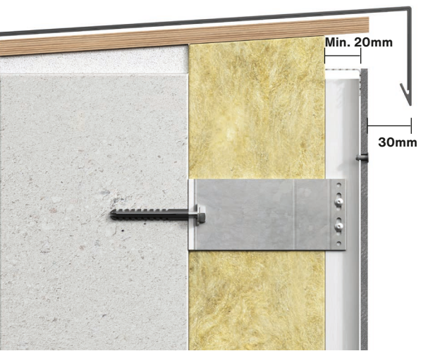
Vertical view: Top construction Make sure that air can move freely from throughout the construction. There should be a minimum free open area of 20mm, or equivalent 200cm 2 per meter to provide adequate ventilation throughout the system. There should be a minimum gap of 30mm between the front face of the facade board and the drip edge of the capping.
