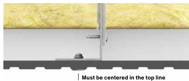
Fig. 2. Swisspearl Patina Inline installation on L profile.
