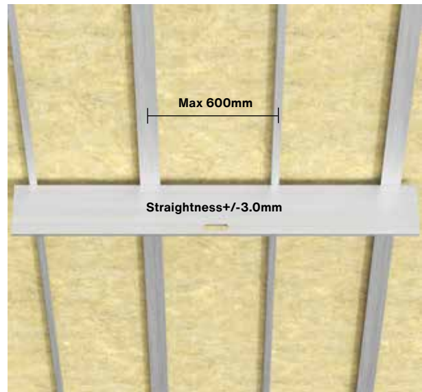
Straightness of substructure
