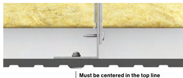
Fig. 2. Swisspearl Patina Inline installation on L profile.
