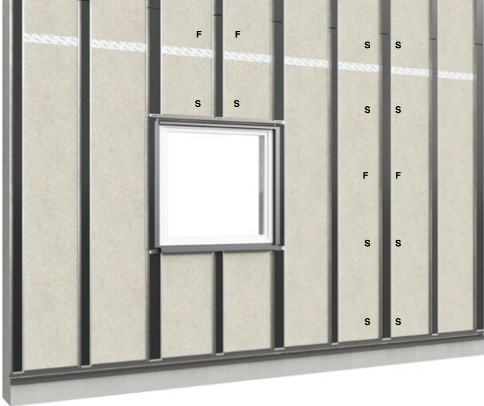
Fixing points (F) Sliding points (S)
