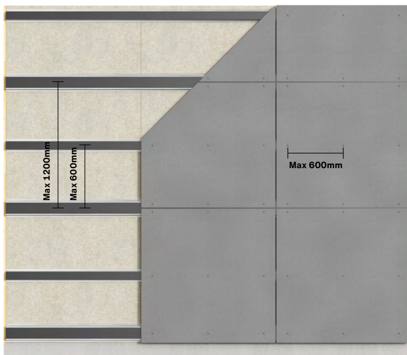
Swisspearl facade boards installed on horizontal VFL profiles
