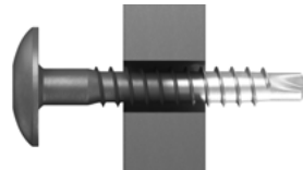
X : Fixing position hole diameter \varnothing 5 mm.
