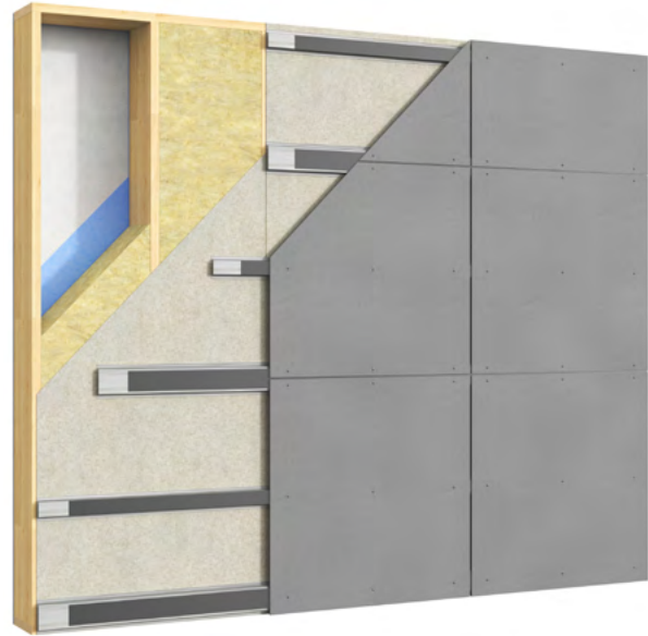
Light wall with horizontal VFL steel profiles
