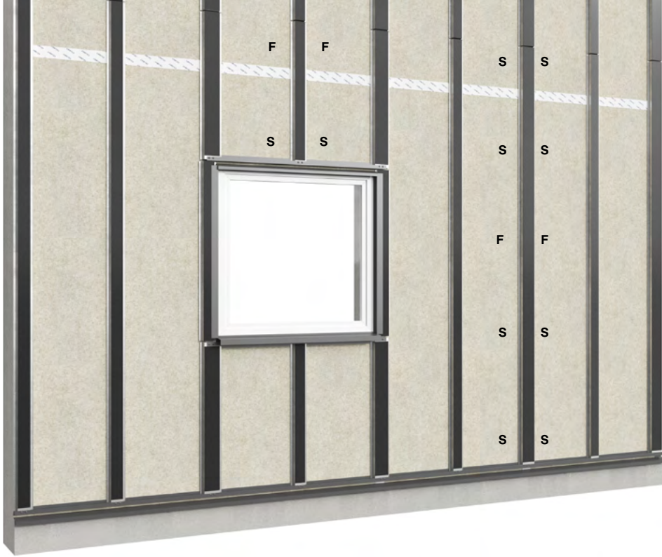
Fixing points (F) Sliding points (S)
