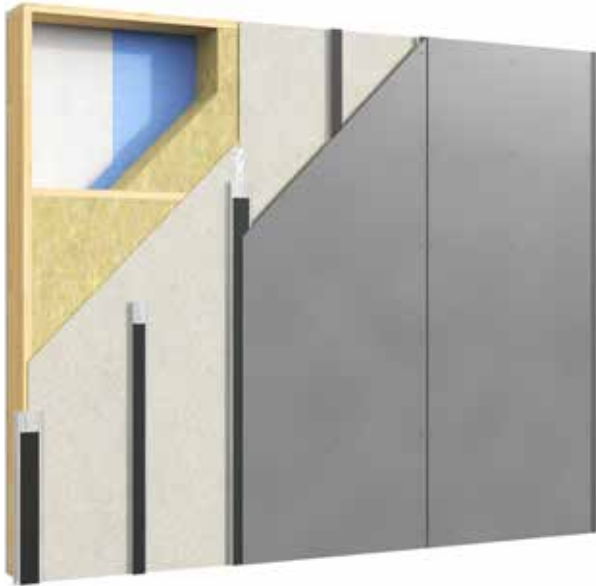
Light wall with vertical VFL steel profiles
