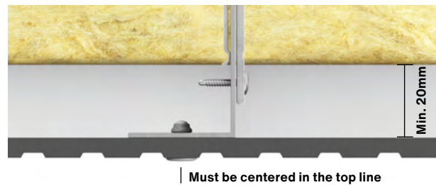
Fig. 2. Swisspearl Patina Inline installation on L profile.
