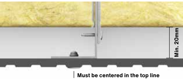
Fig. 2. Swisspearl Patina Inline installation on L profile.
