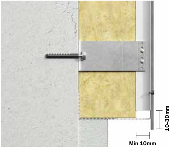
Vertical view: Plinth construction Ensure that the facade boards project past the base of the support from 10 to 30mm, thereby allowing the water from the facade to run off. Use a ventilation grill at the base of the cladding to ensure that insects and vermin cannot enter the construction behind the facade boards. There should be a minimum free open area of 10mm, or equivalent 100cm 2 per meter.
