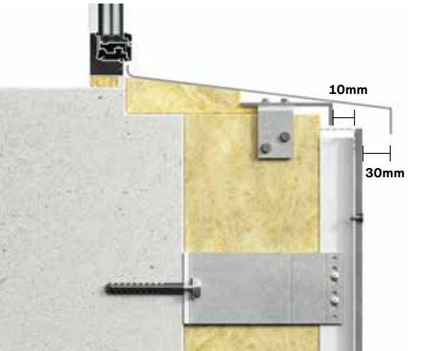
Vertical view: Window Sill Swisspearl facade boards should not be used as sills. We recommend the use of formed aluminium or steel profiles. It is recommended that the sill projects a minimum of 30mm beyond the face of the facade. There should be a minimum free open area of 10mm, or equivalent 100cm 2 per meter between the top facade board and the sill to ensure adequate ventilation behind the facade.
