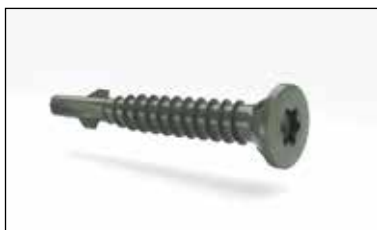
Swisspearl Universal 30 skrūves SCR-S 4,2x30 mm tērauda profi liem (1,2–3,0mm)
