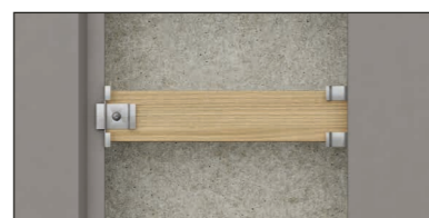
Billede 2 Swisspearl Plank Connect Clips monteret lodret
