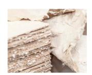
Our fibre cement consists of cement, pulp, water, plastic fibres and air. The combination of these ingredients results in a durable building material that is also lightweight compared to other cement materials. Holding the material reveals its homogeneous nature and surface quality. Its appearance highlights the unique character and natural texture.
