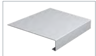
6. Swisspearl Window Sill Profile 25x130mm coloured aluminium external sill profile for horizontal finishing
