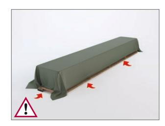
Important: Store materials under a dry and well-ventilated tarpaulin. If the product becomes damp, it should be placed on its vertical edge to allow rapid drying. Never install wet products.
