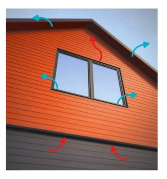
This passage must be a minimum of 15mm in the top and bottom or equal 150mm per m<sup>2</sup>. If grids or similar are used, the openings must equal 150cm<sup>2</sup> per linear meter.
