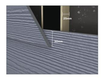
For fast, easy and accurate installation, we recommend using a Swisspearl Gecko Gauge. The Geckos assist in creating the correct overlap and ensure proper location of the screw or nail. Using a Gecko Gauge set clamped to either end of the Planks, makes it possible for one man to install Swisspearl Planks.
