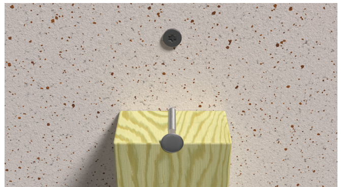
For center battens, ensure that you do not place nails too close to the edge of the underlying structure
