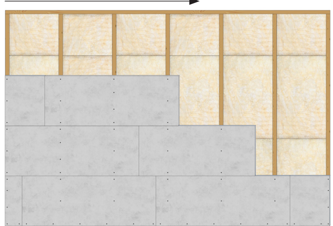
Example of Swisspearl Windstopper Connect with staggered joints
