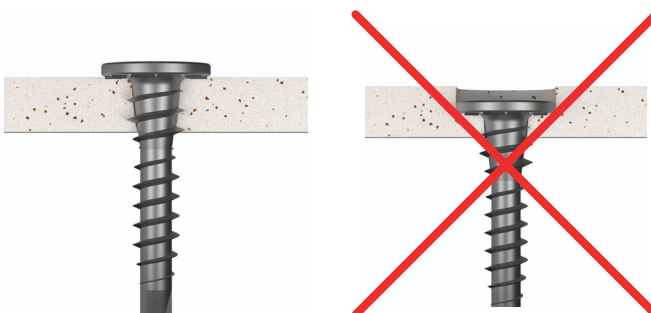
screw installation: Swisspearl Windstopper 4.5 mm
