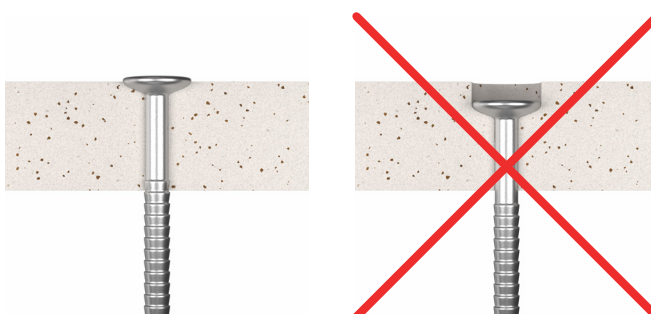
nail installation: Swisspearl Windstopper 4.5 mm and 9.0 mm
