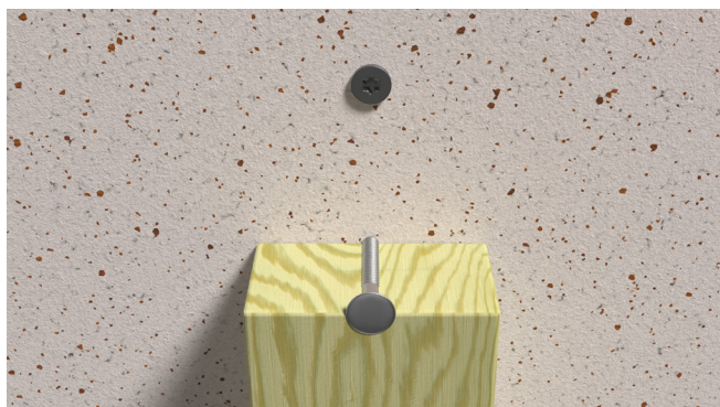
For center battens, ensure that you do not place nails too close to the edge of the underlying structure
