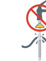
To achieve a watertight and weathertight seal, it is important to confirm that the sealing washer is correctly tightened. Not over tight, not too loose. After a period of time, when the material has settled, the fixings may require re-tightening with hand tools. Be sure to use roof ladders to avoid walking on the roof sheets.
