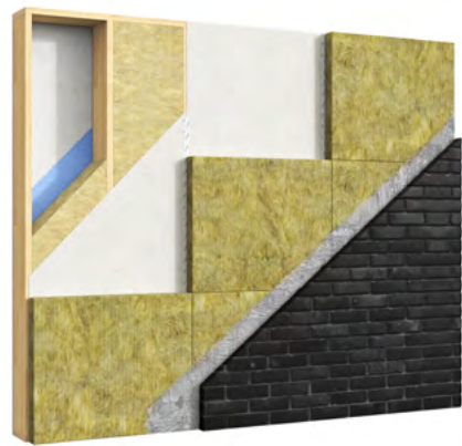
Typical build-up for a structure with Swisspearl Windstopper
